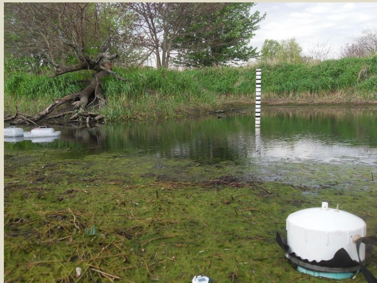
Terrestrial and floating GHG chambers (left). An outlet Agri Drain structure equipped with a V-notch weir, pressure transducer, and data logger (right).
