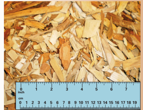
Figure 2. Woodchips commonly used in woodchip bioreactors
